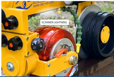
The flaw detector is equipped with special devices that ensure the reliable trajectory of the flaw detector's movement on switches and crosspieces regardless of the direction of movement. This function allows to perform unstoppable testing of all railway track elements.
