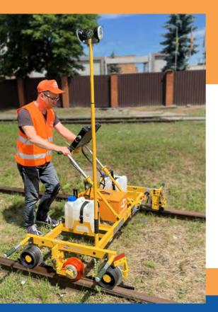
The position of the electronic control and visualization unit (monitor) can be adjusted in three axes. The electronic unit has protection class IP65 according to EN60529
